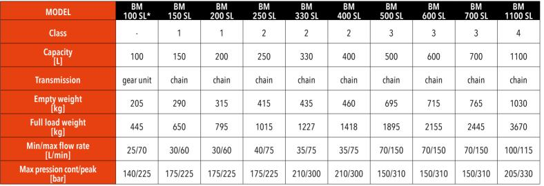
bucket with manual side discharge, without unloading pipe and electro valve
